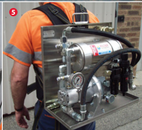
1. Trailer mounted FM42444 bulk fuel filtration unit polishing diesel fuel at Canberra CSIRO tracking station. 2. FM42043 bulk diesel filtration system. 3. Final drive kidney loop filtration. 4. Swing box filtration unit on mining shovel. 5. Portable backpack filtration unit.
