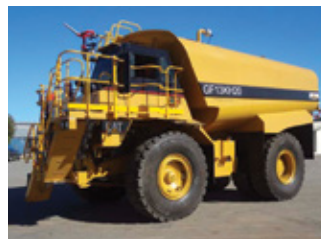
Cat water truck
