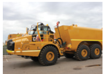
Cat 730 water truck
