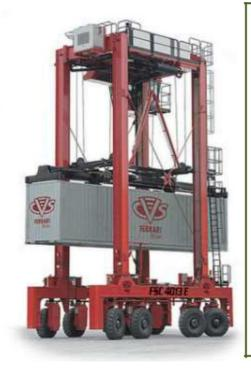
A straddle carrier or straddle truck is a freight carrying vehicle that carries its load underneath by "straddling" it, rather than carrying it on top like a conventional truck. The advantage of the straddle carrier is its ability to load and unload without the assistance of cranes or forklifts. The lifting apparatus under the carrier is operated by the driver without any outside assistance and without leaving the driver's seat.
