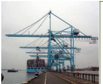
A gantry crane is a crane built atop a gantry, which is a structure used to straddle an object or workspace. They can range from enormous "full" gantry cranes, capable of lifting some of the heaviest loads in the world, Ship-to-shore gantry cranes are imposing, multi-story structures prominent at most container
